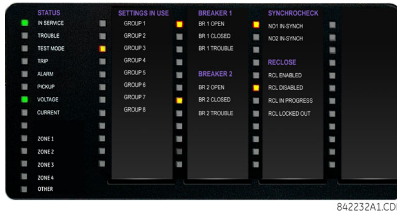
Figure 4-46: B90 LED panel for enhanced front panel
