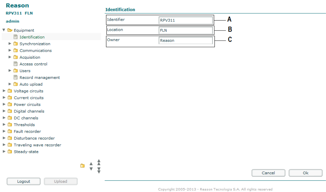
Figure 8: Equipment identification configuration section
