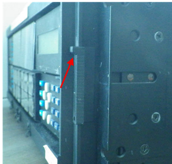
Figure 10-13: Lift latch on standard front panel to open
