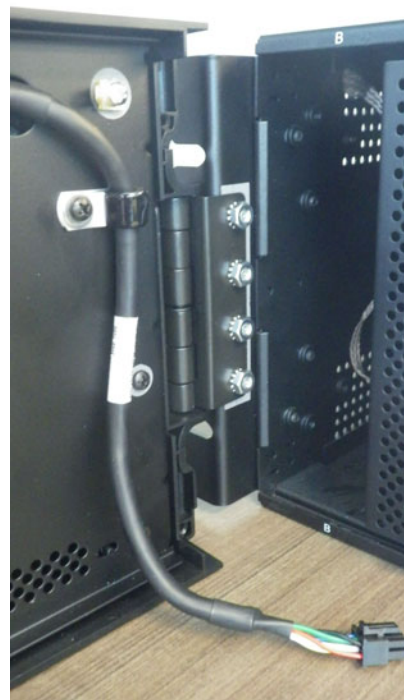
Figure 10-21: Attach to left mounting bracket inside relay
