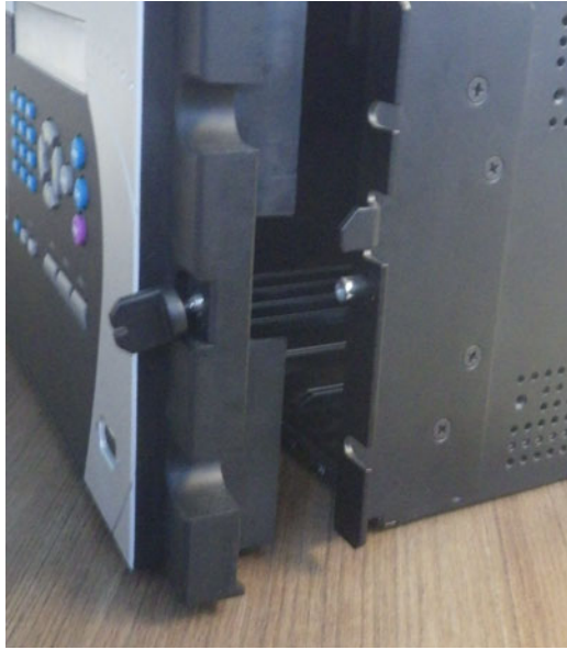
Figure 10-15: Remove standard front panel mounting bracket on right side
