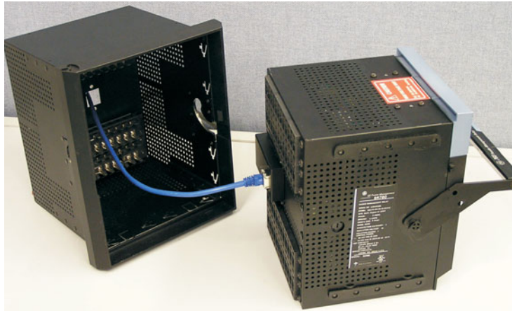
FIGURE 3–10: Ethernet Cable Connection
