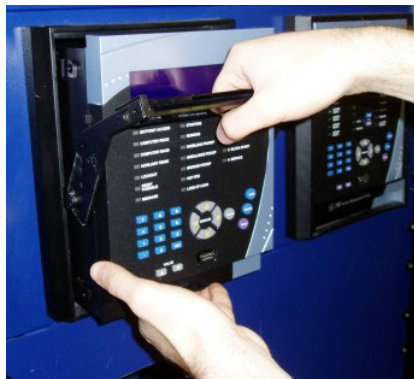
FIGURE 3-9: Slide Unit out of Case
