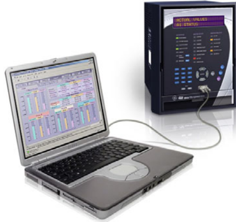
FIGURE 4-2: Communications using The Front RS232 Port
