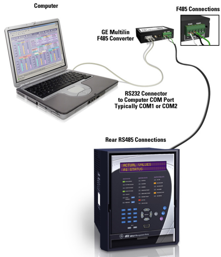
FIGURE 4-3: Communications using Rear RS485 Port
