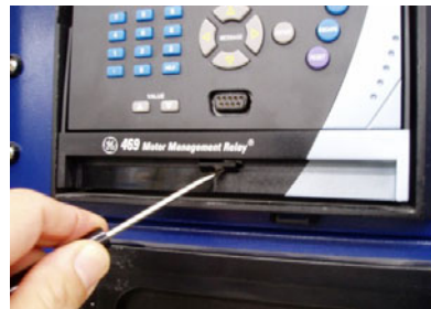
FIGURE 3-7: Press Latch to Disengage Handle
