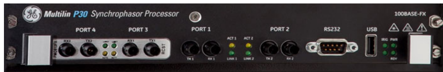
Figure 2-1: Synchrophasor Processor showing 100BASE-FX arrangement
