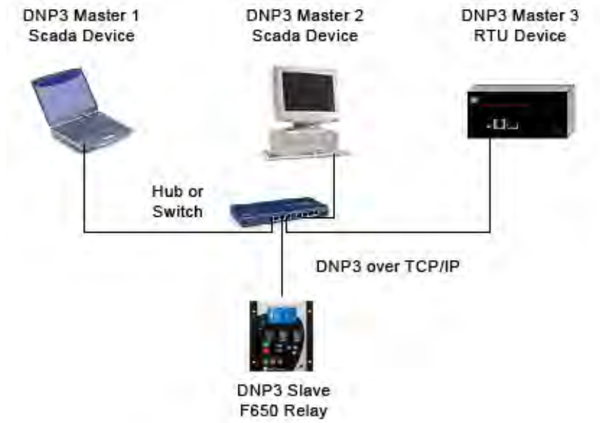
Figure C-3: Multiple DNP3.0 masters communicating with F650
