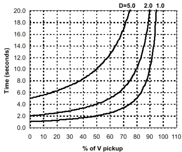
Figure 5-15: Inverse time undervoltage curves
