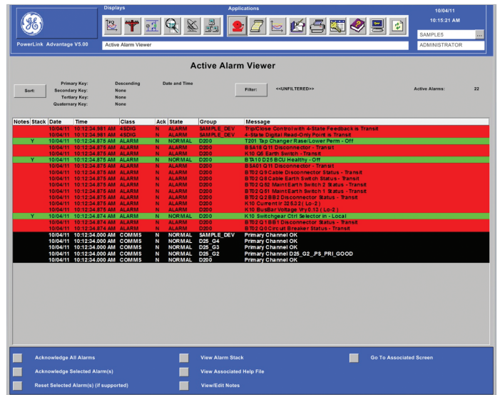
Active alarm viewer to increase operator awareness, decrease response time and improve system reliability
