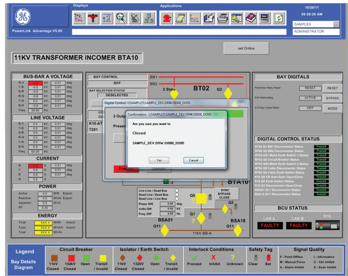
Full SCADA functionality with real-time data acquisition and control
